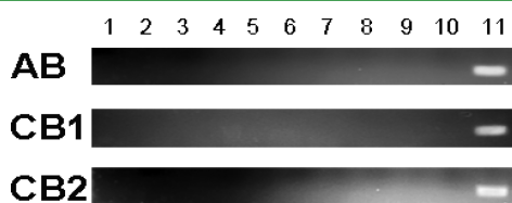
Figure 8. Inhibition of DNA polymerase by adsorption to ASMNPs (primers, QS95-F/-R; DNA templates, Salmonella genomic DNA). ASMNPs:polymerase complexes were prepared by passive adsorption binding (AB); covalent binding using glutaraldehyde as a coupling agent (CB1); covalent binding using EDC as a coupling agent (CB2). The amount of ASMNPs:polymerase complexes: lane 1–10, 5, 10, 20, 30, 40, 50, 60, 70, 80, or 160 \mu g; lane 11, lane 5 with an additional 1 U of Taq DNA polymerase.
